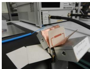
Figure 3: IPC-TM-650 2.5.5.5C clamped stripline test fixture. The two 1.5 mm fully etched coupons are inserted on either side of the patterned resonator card and the fixture is closed to form a stripline circuit
