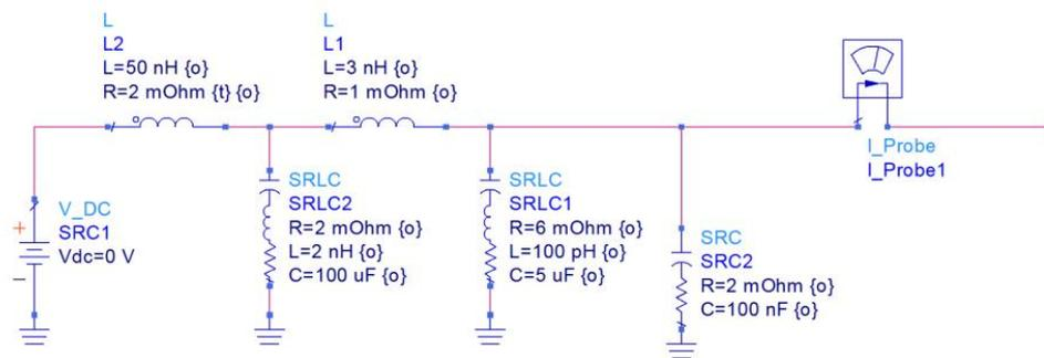
Three resonances, each with a peak impedance of 125mΩ
