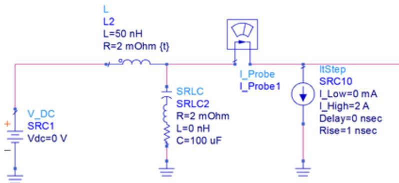
Single resonant circuit with a “target impedance” of 125mΩ is used to demonstrate the voltage response to a fixed dynamic current amplitude
