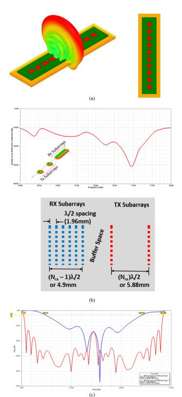
Fig. 3. (a) Sub-array modeled geometry with ANSYS HFSS [12] and simulated 3D polar total gain, (b) Sub-array antenna reflection coefficient and TX/RX subarrays configurations, (c) Far field gain pattern with vertical and horizontal beam-width at 76.5GHz.
