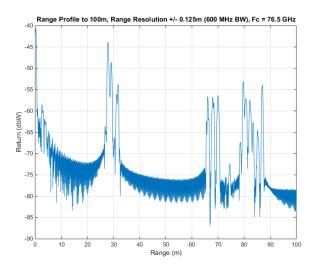
Fig. 6. Radar Range profile and scattering centers.
