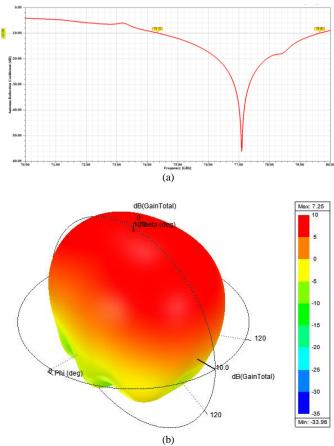
Fig. 2. (a) Proposed patch antenna reflection coefficiet, (b) far field 3D polar gain plot.
