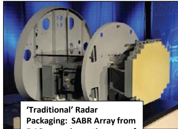
'Traditional' Radar Packaging: SABR Array from F-16, occupies entire nose of aircraft (Photo courtesy Northrop Grumman)
