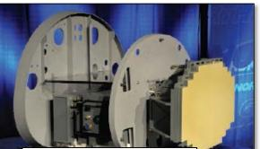
'Traditional' Radar Packaging: SABR Array from F-16, occupies entire nose of aircraft (Photo courtesy Northrop Grumman)
