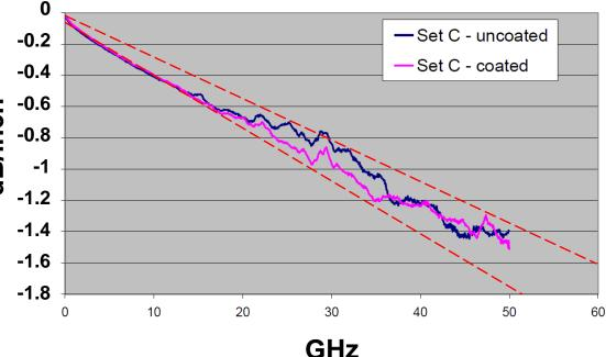
Insertion Loss of 50 Ω Microstrip on 0.0047" Rogers RO4350B Laminate (Red lines show approx. limits of reproducibility in RF measurement)
