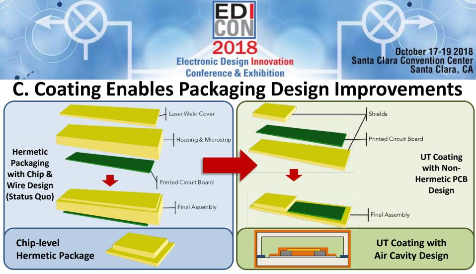
RF-compatible ultra-thin vapor deposited coatings allows RF systems designers to use printed circuit board technology
