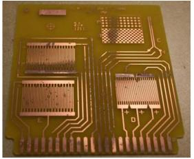
Images of coated board (1  $\mu$ m thick coating) with lower contacts masked and an uncoated board after Salt Fog testing per MIL-STD-810G Method 509.5
