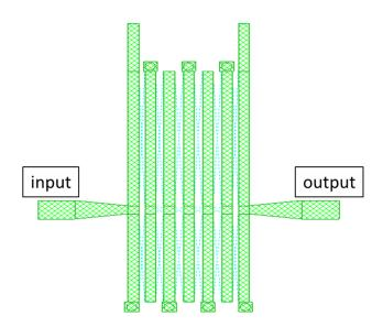
Fig. 4. Layout of the Highband section.
