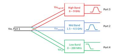
Fig. 1. Block Diagram of a parallel-connected triplexer
