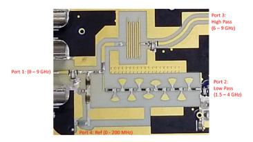
Fig. 7. Fabricated Triplexer.
