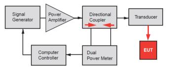
Figure 1: Conducted Immunity Test Setup
