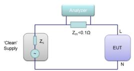
Figure 5: Harmonics Current measurement circuit.
