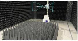
Figure 7: Semi-Anechoic Chamber
