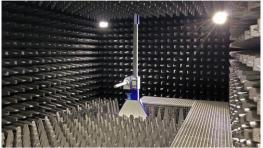
Figure 8: Full-Anechoic Chamber
