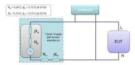
Figure 6: Flicker measurement circuit.
