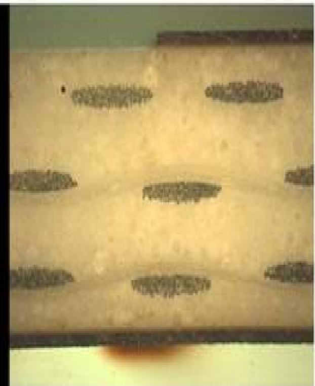
Cross-section of a microstrip
