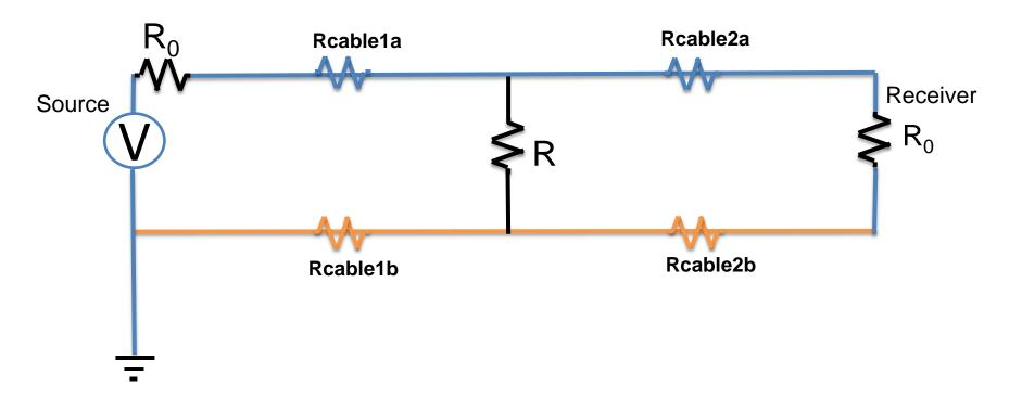
Even if Rcables > R, the measurements are accurate as long as Rcables << R<sub>0</sub>
