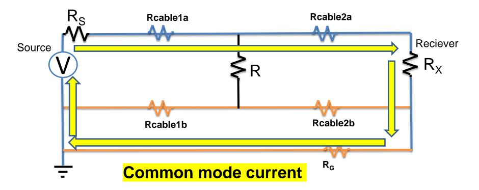
Reduce the common mode current due to the ground loop without affecting safety
