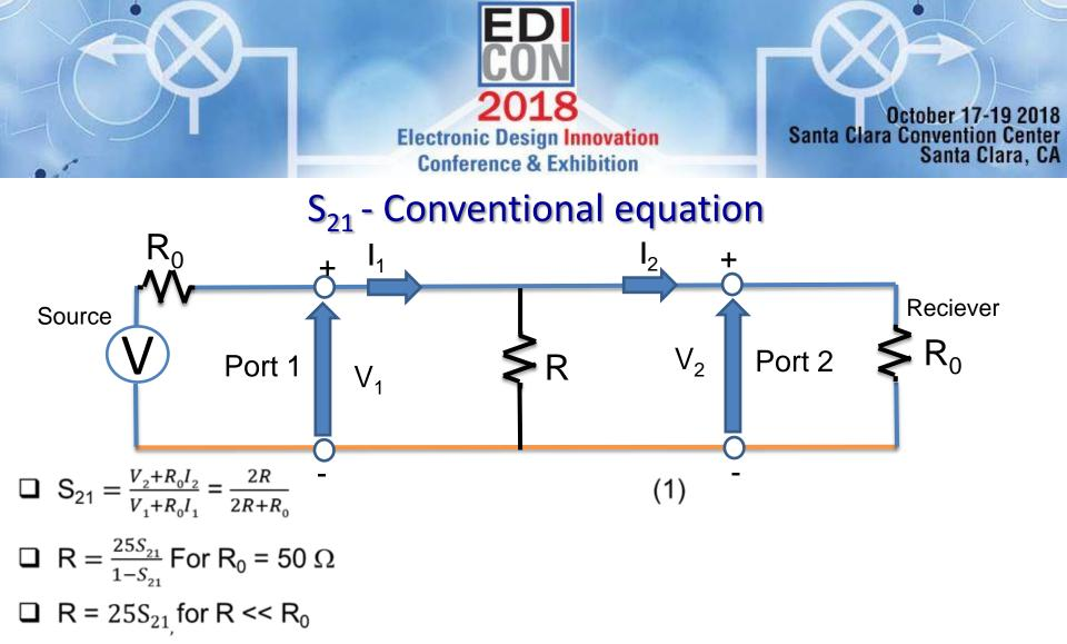
Equation (1) is the commonly used one, but less intuitive impedance (R) measurements
