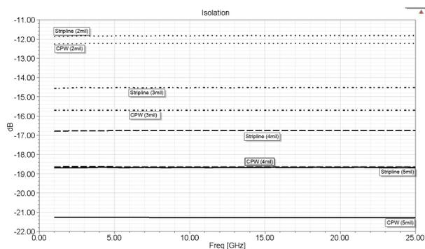
Fig. 9. Isolation for two broadside-coupled CPW lines.
