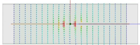
Fig. 2. Vector representation of parasitic slotline (odd) mode.
