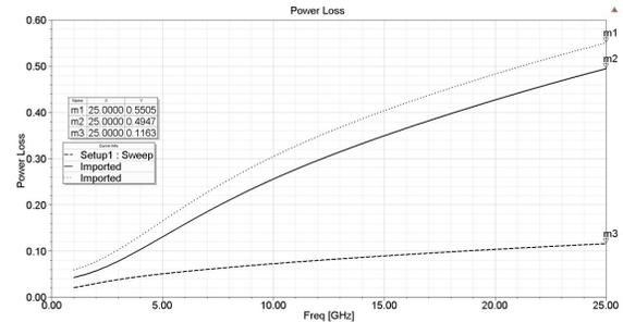
Fig. 3. Contribution of losses to CPW loss. (a) ohmic losses (b) ohmic and dielectric losses (c) ohmic, dielectric and roughness.
