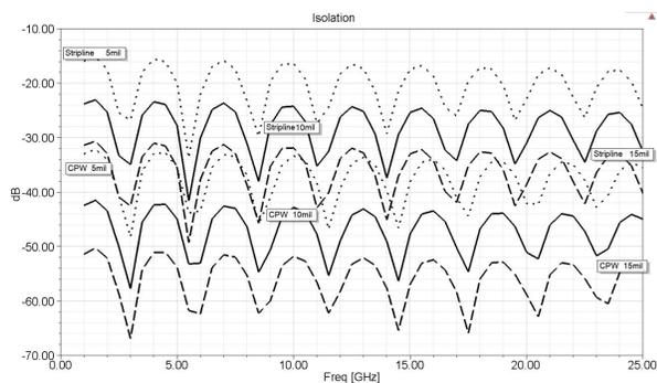
Fig. 6. Isolation comparison for two edge-coupled CPW and striplines.
