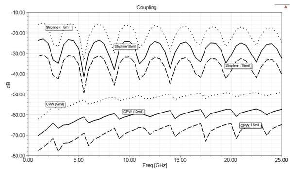
Fig. 7. Coupling for two edge-coupled striplines.
