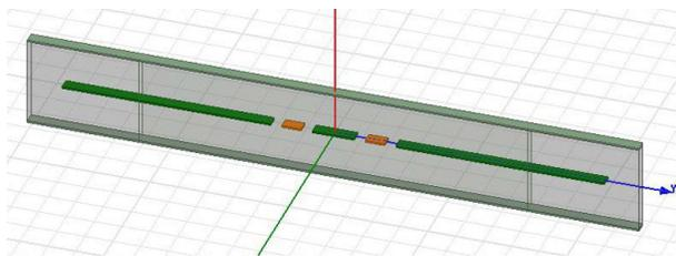
Fig. 5. Edge coupled CPW lines.
