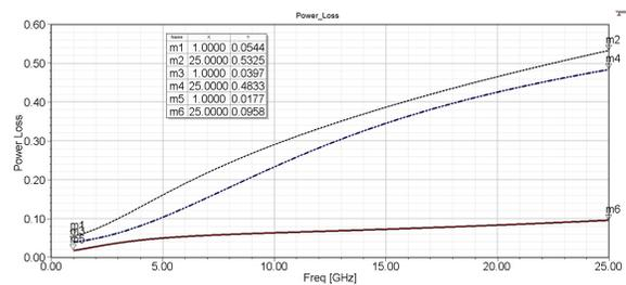
Fig. 4. Contribution of losses to CPW loss. (a) ohmic losses (b) ohmic and dielectric losses (c) ohmic, dielectric and roughness.
