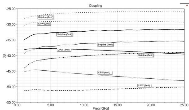
Fig. 10. Coupling for two broadside-coupled striplines.
